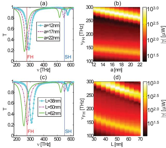
FIG. 4: (a) Linear transmission spectrum and (b) nonlinear mode overlap  $|\gamma|$  for cap detuning. Likewise, (c) and (d) show the linear transmission and mode overlap when the length of the antenna is detuned. The nonlinear mode overlap is obtained by illuminating with a pump of power 1W per unit cell. Please note that  $|\gamma|$  is shown on a logarithmic scale.
