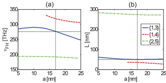
FIG. 3: (a) Pump frequency  $\nu_{\text{FH}}$  and (b) length  $L$  for the given cap radius  $a$  where double resonance is possible for FP orders  $m, n$  at FH and SH respectively. Horizontal and vertical black lines indicate the operating configuration ( $\nu = 276$  THz,  $a = 17$  nm and  $L = 50$  nm) chosen in this study.
