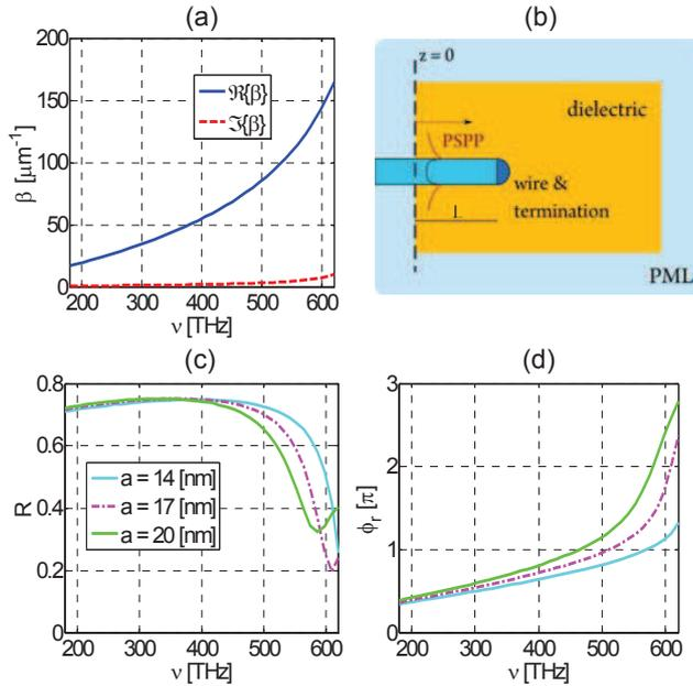
FIG. 2: (a) Dispersion of fundamental  $\text{TM}_0$  mode computed for a cylindrical wire of radius 15nm. (b) Schematic illustration of the 3D geometry used for obtaining the modal reflection coefficient  $r(a, \nu)$  of  $\text{TM}_0$  mode. (c) Squared amplitude  $R(a, \nu) = |r(a, \nu)|^2$  (c) and (d) phase  $\phi_r(a, \nu) = \arg[r(a, \nu)]$  of the reflection coefficient are also shown.
