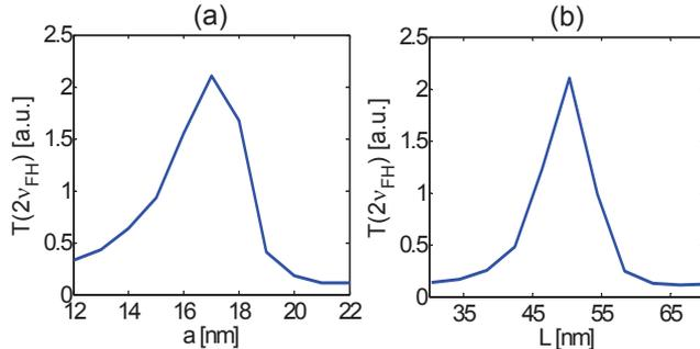
FIG. 5: (a) Transmission spectrum of nonlinear FDTD simulations when illuminated with a CW pump of power 13mW at  $\nu = 277\text{THz}$  showing the effect of detuning the cap radius  $a$  where  $L = 50$  nm(a) and (b) length  $L$  where  $a = 17$  nm from their resonant values of  $a = 17\text{nm}$  and  $L = 50\text{nm}$ , respectively.
