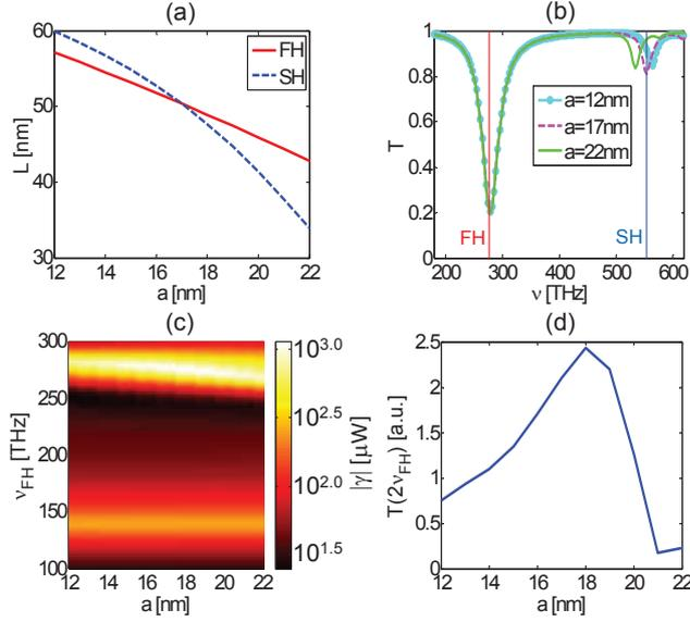
FIG. 6: (a) Antenna configuration at  $\nu_{\text{FH}} = 277\text{THz}$  when FH has FP resonance of 1<sup>st</sup> and SH of 3<sup>rd</sup> order. (b) Linear transmission spectrum and (c) nonlinear mode overlap  $|\gamma|$  are shown when the antenna is kept resonant at FH according to (a). Likewise, the transmission spectrum of nonlinear FDTD-simulations is shown in (d) when the structure is illuminated with a pump of  $\nu_{\text{FH}} = 277\text{THz}$ .
